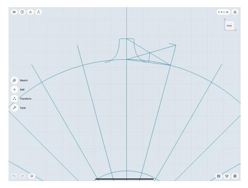
I set up a construction plane. With 15 degrees spacing for a 24 tooth ring. Most chainrings and sprockets are even spacing.
