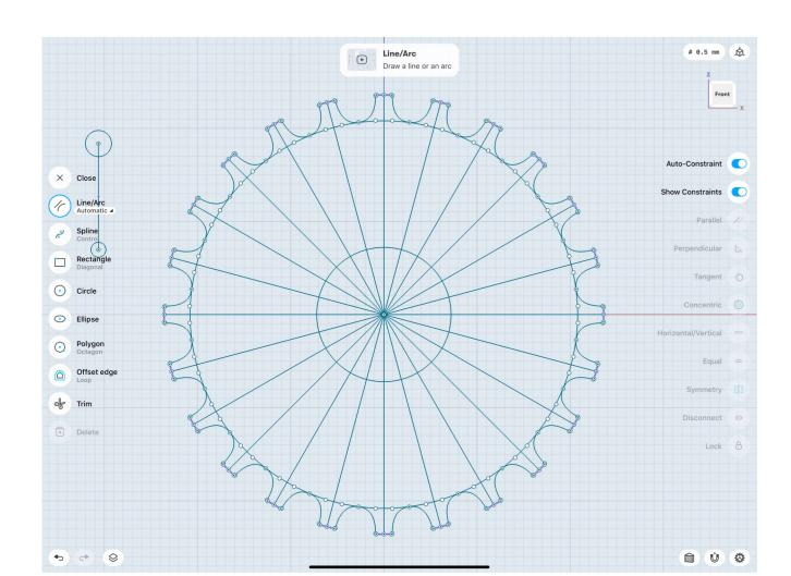
I extruded the radial tooth shape from the profile disc creating the main shape. I then added multiple Boolean extrusions to create the internal details.
